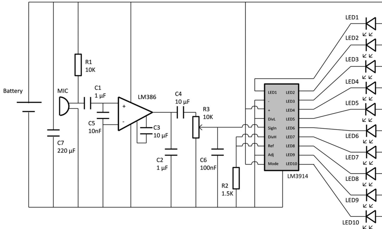
The sound meter circuit uses a microphone to detect sound and then uses a number of LEDs to indicate the how loud the sound is.
