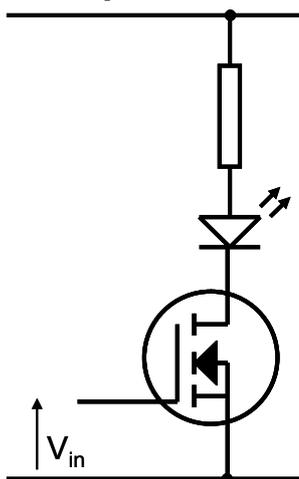
In this circuit an FET is connected to an LED, however it could be used to drive any load including higher power loads. When  $V_{in}$  is at zero volts the gate of the FET has no voltage on it, and no current flows through the LED. When  $V_{in}$  is high the FET turns on and current flows through the FET from the drain to the source and the LED lights.
