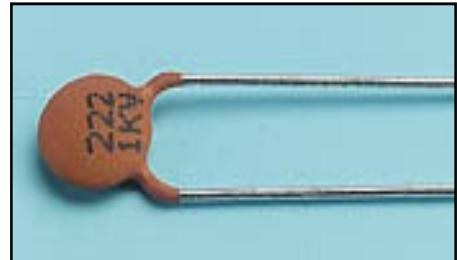
Example:  $104 = 10 + 0000$  (4 zero's) = **100,000 pF** (which is also  $0.1 \mu\text{F}$ )
