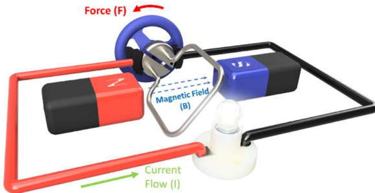
When the generator shaft is turned the coil moves. From moving the coil in the magnetic field a current is created. The current flows round the coil and out of the commutator. The current moves in accordance with Flemings Right Hand Rule.
