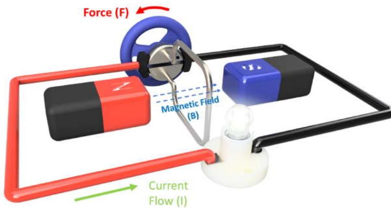
As the coil rotates towards the opposite side the current would change direction.
