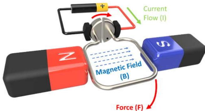
When a voltage is applied (via the commutator) current flows around the coil. A force is created from magnetic field, and the coil moves away in accordance with Flemings Left Hand Rule.
