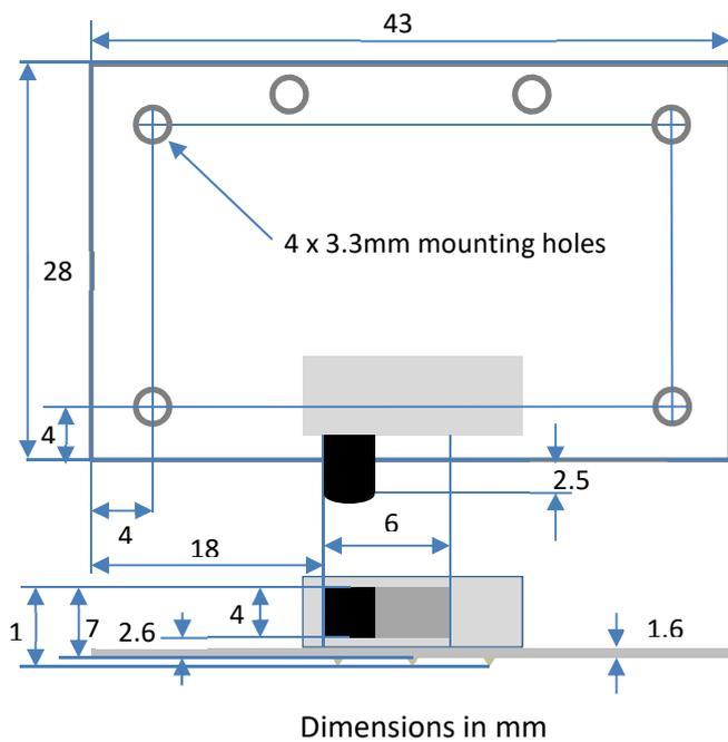
The four mounting holes are all 4mm from the board edge.
