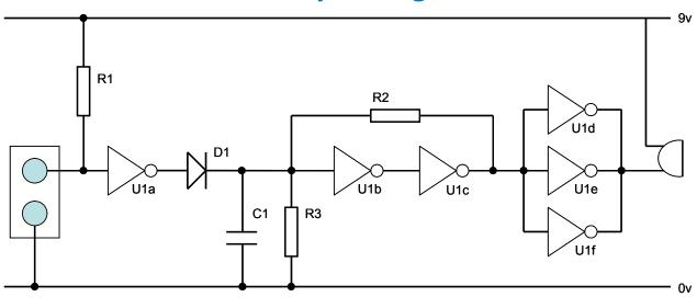
The connections to the wire are shown on the left of this diagram. When the two are joined there will be a resistance across the connections made by the body. Resistor R1 is a 10M resistor and this normally holds the input to the not gate (U1a) in a high state. When the connection is made across the input, which will be in the order of a few hundred  $K\Omega$ , the input to the not gate (U1a) will be low.
